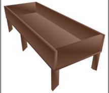
The flange also ensures that there will always be some water left in the tank (about half an inch) to prevent the black plastic from melting. It also will maintain very hot water that will help to heat up any fresh cold water put into the tank.
