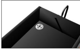
Take a piece of 4 to 6 mil black plastic and lay inside the enclosure with excess you can cut off later. In a corner of the enclosure, most convenient to running feed line to the hot water tank, drill a hole just big enough for the pipe you are using. Just cut a
